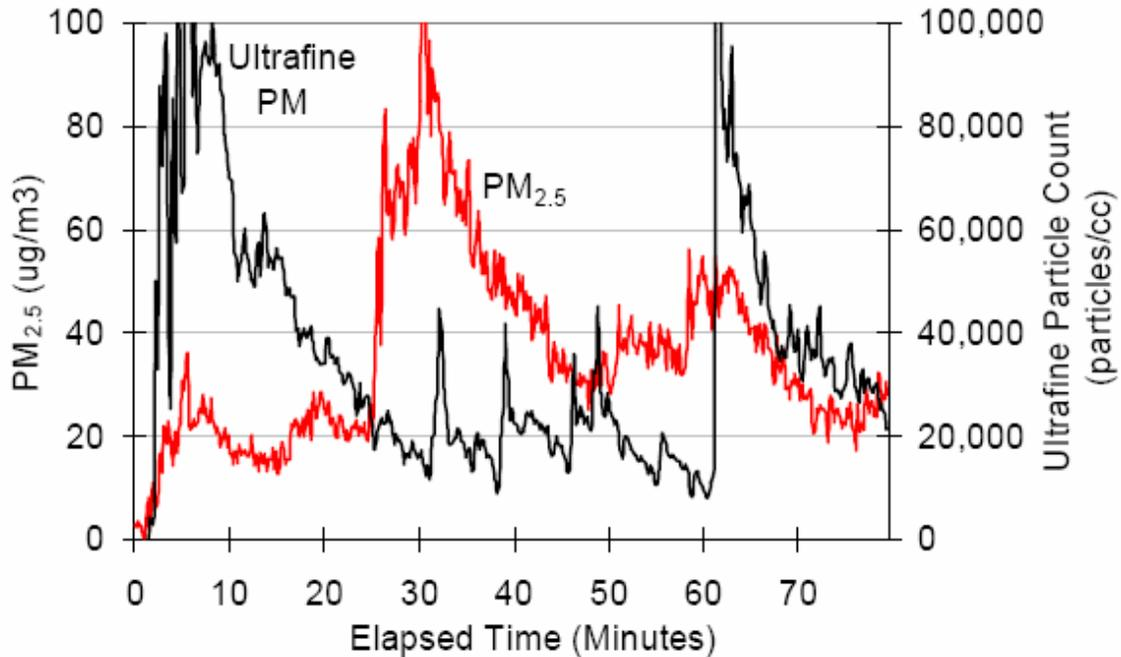
**Figure 1: Conventional buses tested showed significant  $PM_{2.5}$ , ultrafine particle, black carbon and PAH self-pollution. (Ambient concentrations have been subtracted.)**
