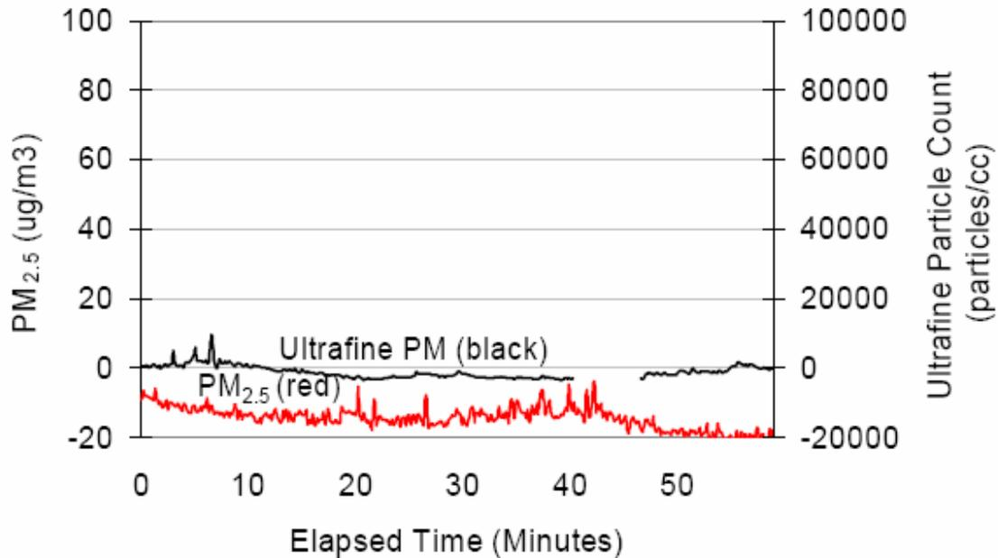
**Figure 2: The DPF-ULSD-Spiracle combination eliminated PM<sub>2.5</sub>, ultrafine particles, black carbon, and PAH self pollution from the bus cabin. Ambient concentrations have been subtracted resulting in slightly negative apparent net concentrations. Concentrations below zero should be taken as zero net PM<sub>2.5</sub> contribution to the bus.**
